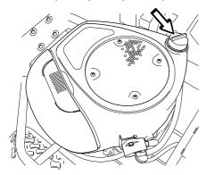
Now insert the dipstick again. The dipstick should be completely screwed down
