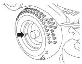
CAUTION! Different tyre pressures on the front tyres will result in the blades cutting the grass at different heights. Having the same air pressure in the tyres is important in order to achieve the best possible performance as well as to avoid damage to the machine
