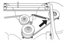
9 Simply reverse the procedure to fit the new belt.
