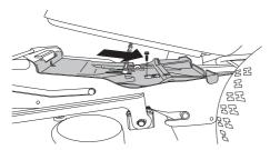
3 Undo the nuts on the lift strut.
