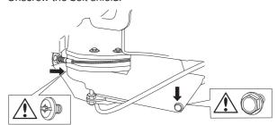
Lubricate using a grease gun, 1 nipple from the right-hand side under the engine's lower belt pulley, until grease is forced out. With daily use, lubrication should be carried out twice weekly.
